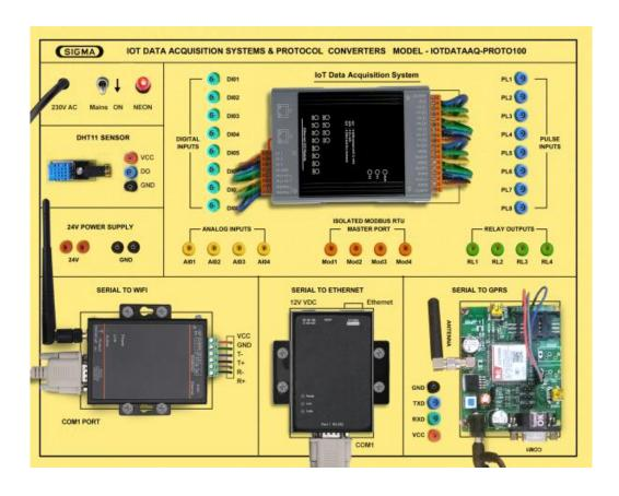
This trainer has been designed with a view to provide practical and experimental knowledge of Data Acquisition Systems & Protocol Converters.
